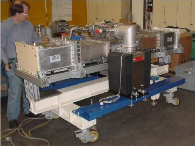
Figure 7: Two 500 MHz waveguide windows assembled for RF processing [22].
