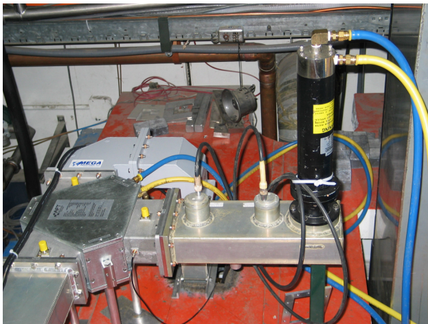
Figure 4: 20 kW CW AFT circulator with RF load.
