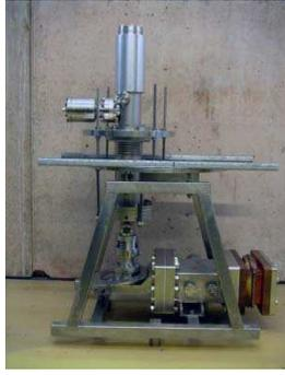
Figure 2: Coupler stand used for warm coupler tests.
