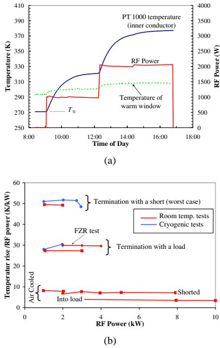
Figure 4: (a) Example of PT1000's temperature versus time. Measurements were made with HOBICAT cold and the waveguide shorted. (b) Summary of the all tests.
