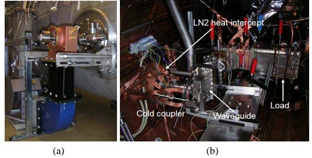
Figure 3: (a) Warm part of the coupler mounted on the outside of HOBiCAT. (b) Cold part of the coupler mounted in HOBiCAT along with the waveguide load. The copper straps are used to cool the 77-K and 2-K points of the coupler to about 100 K.
