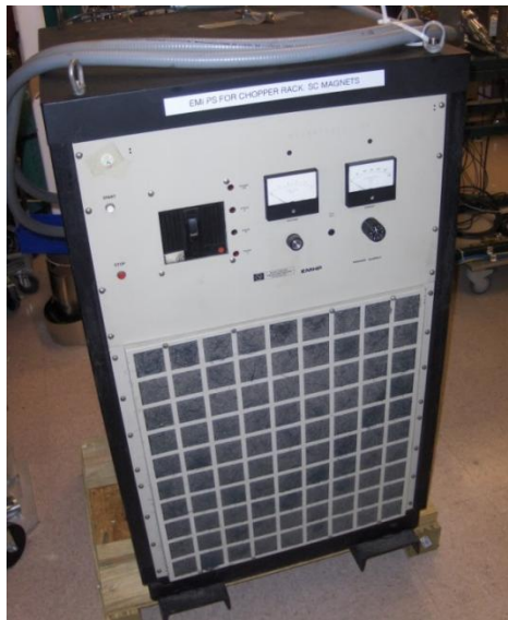
Figure 15. Old fashion PS used for feeding the current sheets; able to generate 3 kA. In sheets
