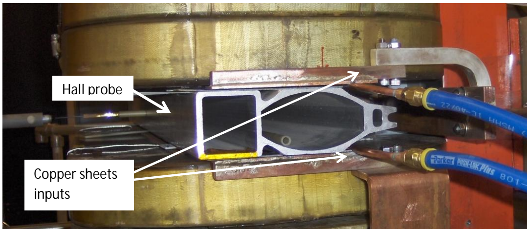
Figure1. Two insulated~3mm-thick current sheets inserted in the gaps between the vacuum chamber and the upper and lower poles. The sheets are running along the magnet poles. Hall probe is moving across the chamber in the middle through the holes drilled in the walls of chamber. Water cooling tubes (blue ones) feed the water cooling tubes brazed to the sheets at the side edges.
