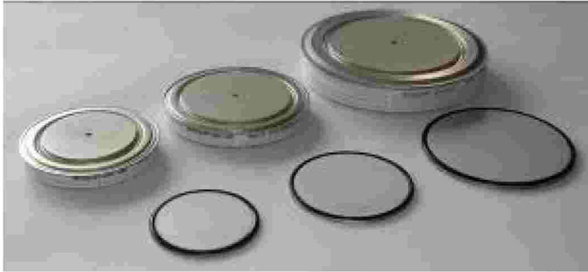
Fig.2. Reverse – switched diodes for peak current from 200 kA to 500 kA and blocking voltage of 2400 V, encapsulated in hermetic metal – ceramic housing and without housing (RSD sizes of 64, 76, and 100 mm)
