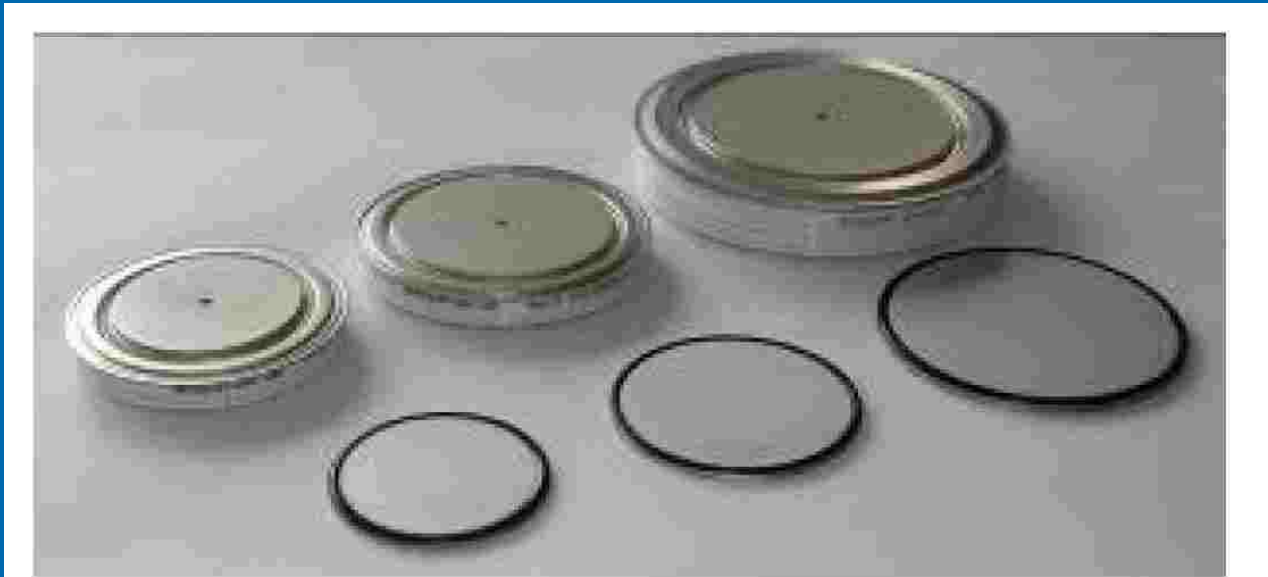
Fig.2. Reverse – switched diodes for peak current from 200 kA to 500 kA and blocking voltage of 2400 V, encapsulated in hermetic metal – ceramic housing and without housing (RSD sizes of 64, 76, and 100 mm)
