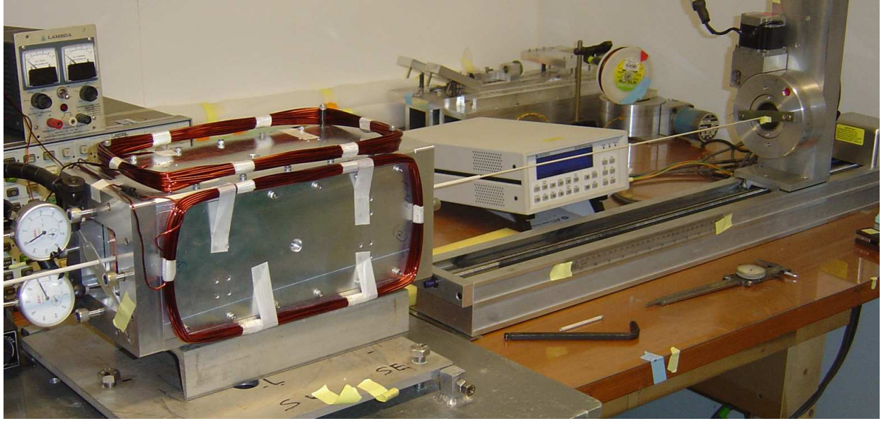
FIG. 4: Magnetic field measurement bench with the tested "Delta" undulator model. The seen are: background field compensating coils; ceramic tubing guiding Hall probe through the undulator bore; screws used for magnet array displacement.
