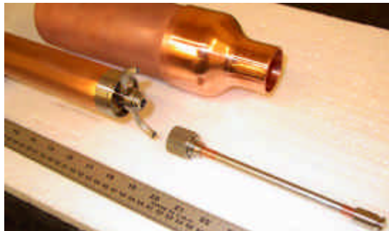
Figure 5: Cold mass, transition to the room temperature flange, part of 70 °K shield.
