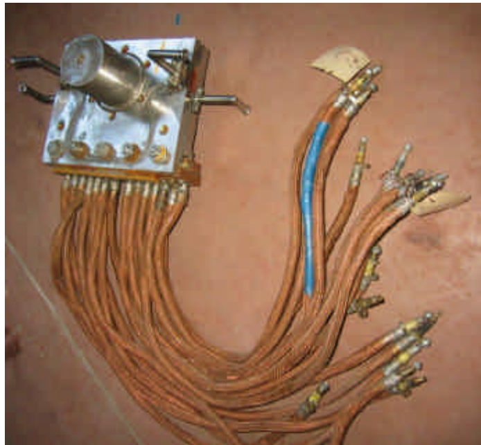
Figure 18: Lithium lens with feeding cables connecting lens with secondary windings of a transformer. (Courtesy of Yu. Shatunov, BINP).
