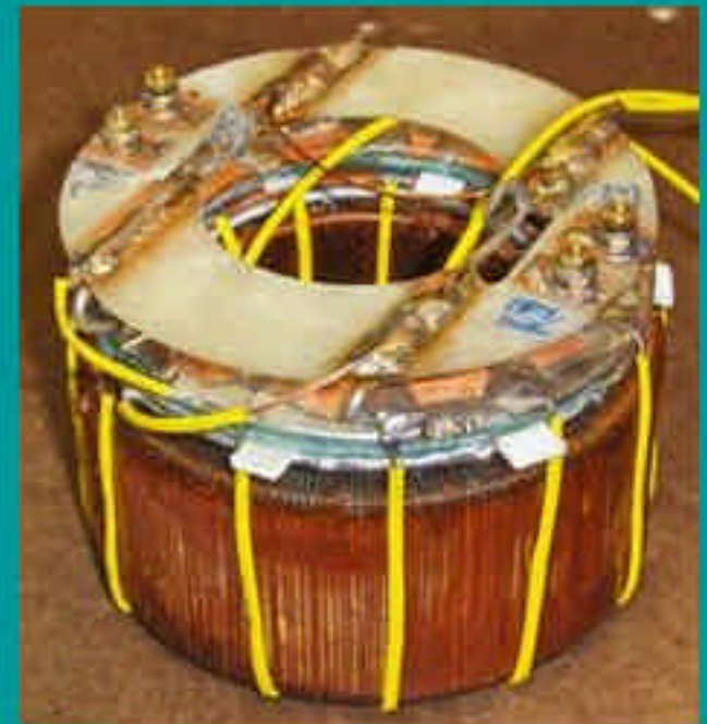
SC transformer with keys
