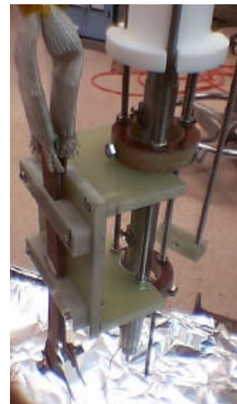
Figure 26: Undulator having a period of 10 mm and aperture 6mm develops K \cong 0.33 for I=200A . Tube diameter is 6 mm. Tested up to 400 A.
