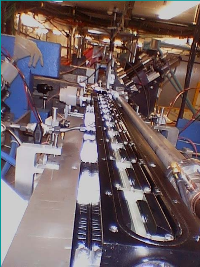
Undulator installed in FFTB
