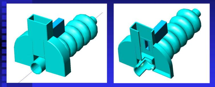
HOM evacuation waveguide made with reduced width, this prevents the leakage of RF power there. High order modes, having higher frequency, escape through this waveguide.
