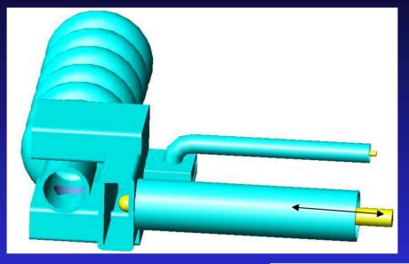
Now as the coaxial has no direct view to the beam, it is possible to use it for coupling tuning.
