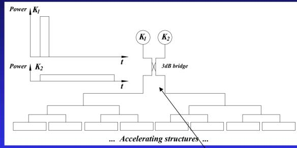
At the beginning the power excides the one required for the steady beam acceleration;
