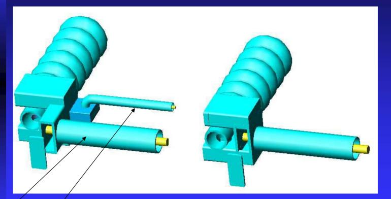
Main pówer HOM coax At the right -the holes are shifted azimuthally, the same coaxial used for evacuation of HOM
