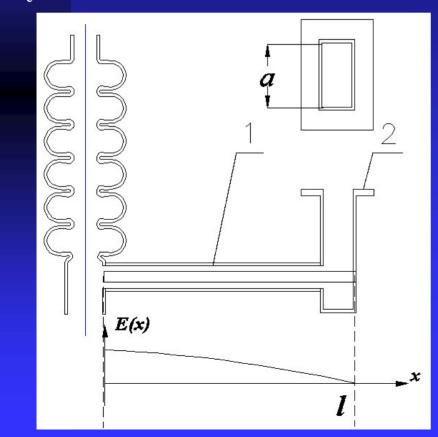
This means that part of the transmission line between the orifice looking to the beam and the coax-waveguide transition can trap RF waves with a spectrum within the bandwidth  $\{0-\pi c/a\}$ .
