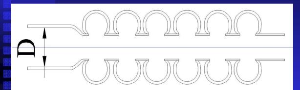
What is important here is that diameter **D** of the tube is chosen so that the transverse mode can propagate inside, i.e. its diameter,  $D \ge Dcr = \lambda_{tr}/1.81$  where  $\lambda_{tr} = c f_{tr}$
