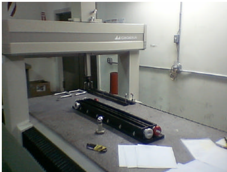
Figure 11: Test of dimensions with coordinate machine.
