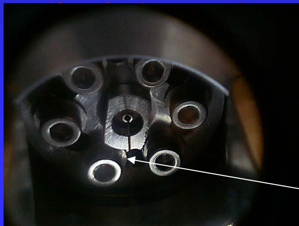
Stretched wire for aperture measurements
