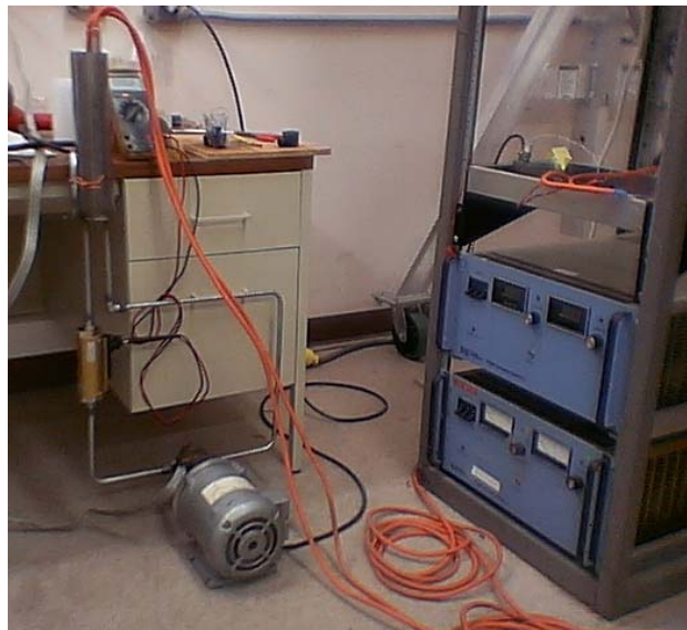
FIGURE 5: Pump, flow meter and reservoir make the loop for investigating FF flow. Sample coil made with wire 0.6 \times 0.6 \text{ mm}^2 and immersed in flow feed by power supply, right, up to 70 A.
