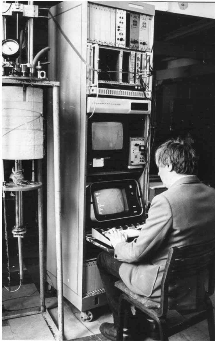
Fig.38. General view to the equipment under preparation for test of superconducting undulator.
