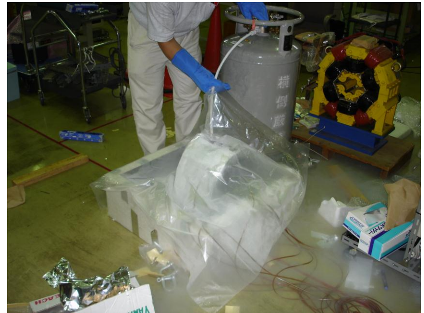
Liq. N 2 was poured into the tank not to splash directly
