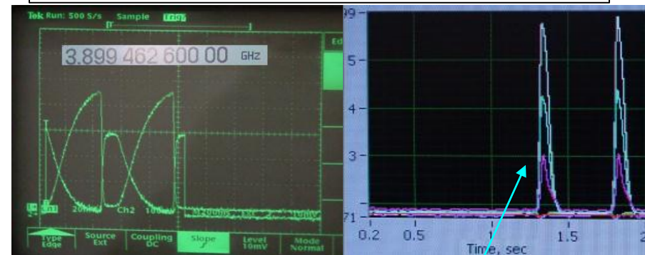
QvsT at Pi-mode. F=3899.46 MHz. Cavity baked 150C 48 h. Rres=25 nOhms.
