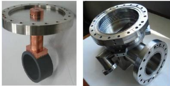
Figure 3: parts of the BLA prototype: (left) damping ceramic ring welded to the copper stub and (right) housing made of stainless-steel.
