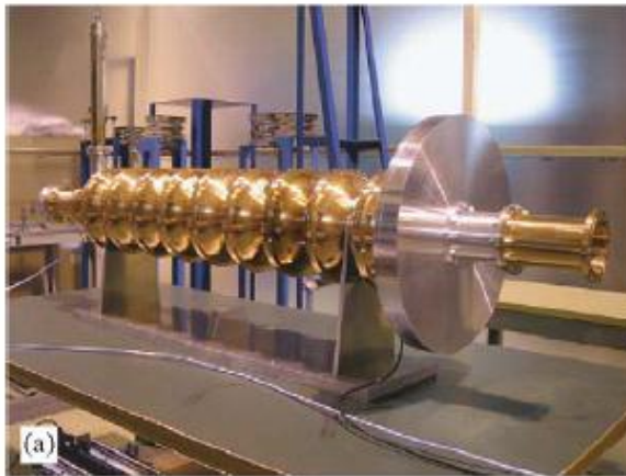
Fig. 2. (a) Low-power model of a 9-cell TESLA type cavity equipped with a radial-line HOM damper and (b) inside the radial-line HOM damper.
