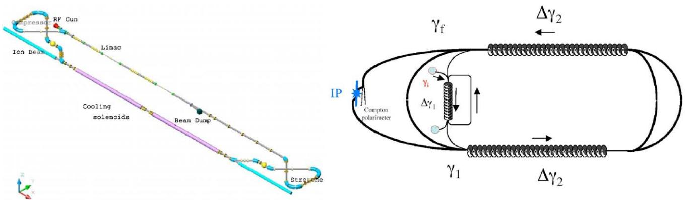
Fig. 4. Layout of an ERL for electron cooling of RHIC's ion beam and of the ERL that would provide electrons for collisions with the RHIC polarized proton and ion beams.
